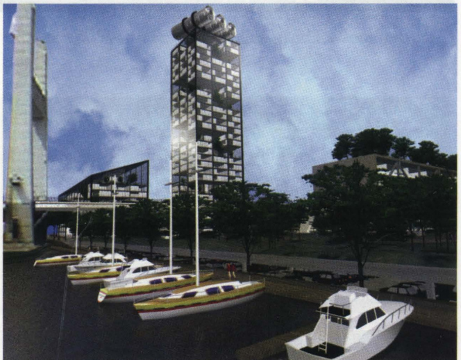
View from the marina. Three wind tunnels on top of the building provide energy for the whole complex.
